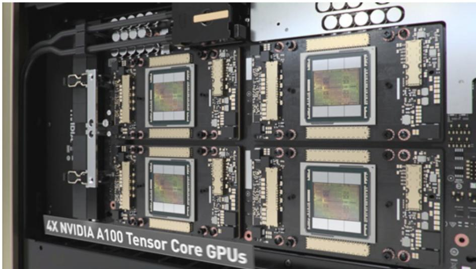
Figure 9. View of the 4-way NVIDIA HGX board inside NVIDIA DGX Station A100.
