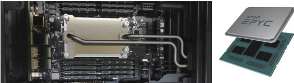
*Figure 13. View of the AMD Epyc 7742 processor, covered by its cold plate.*
