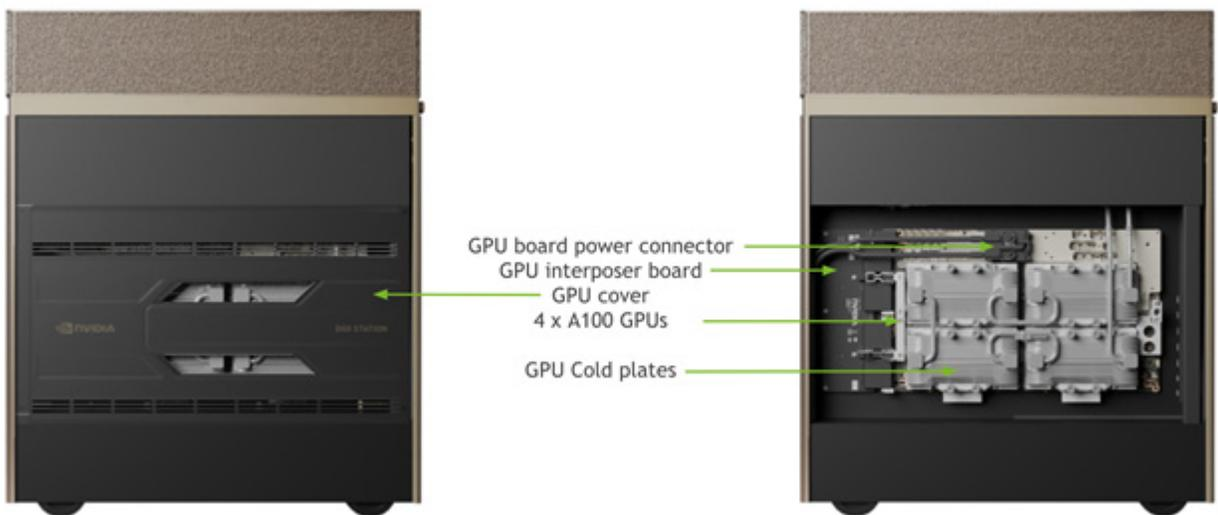
Figure 10. View of NVIDIA DGX Station A100, GPU side, with GPU cold plates.
