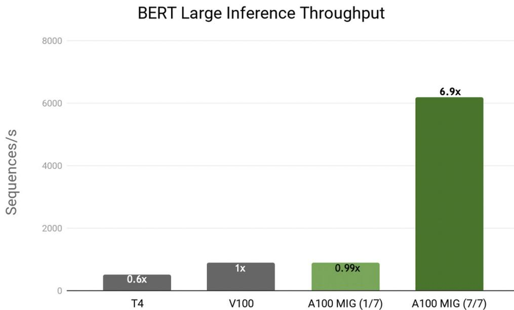
*Figure 7. Up to 7X Higher Inference throughput with Multi-Instance GPU (MIG). Above results were performed on a DGX A100. BERT Large Inference (with Sequence Length=128)*
