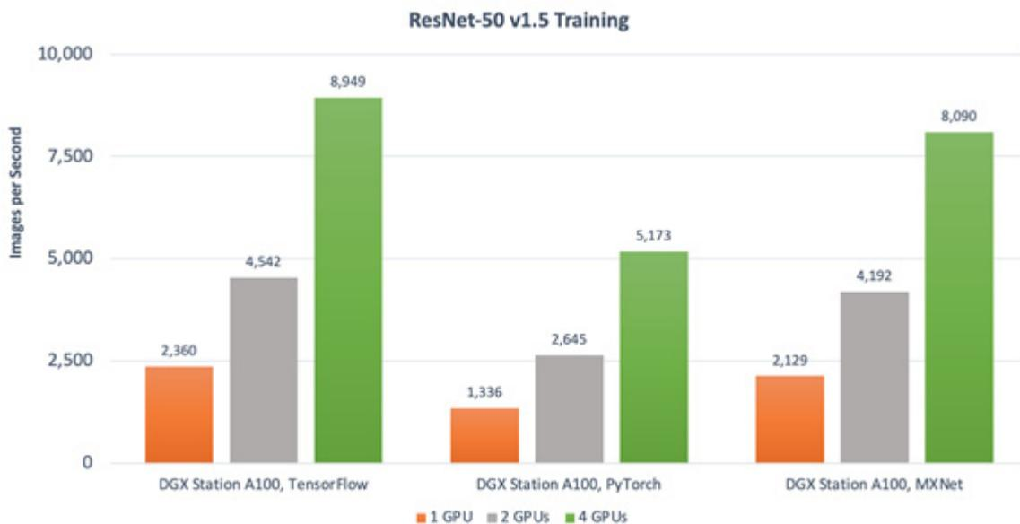
Figure 20. DGX Station A100 (4x A100 SXM 80GB), ResNet-50 V1.5 training, Mixed Precision, TensorFlow (21.02-tf1\_py3, bs 256), PyTorch (21.02\_py3, bs 256), MXNet (21.02\_py3, bs 192)
