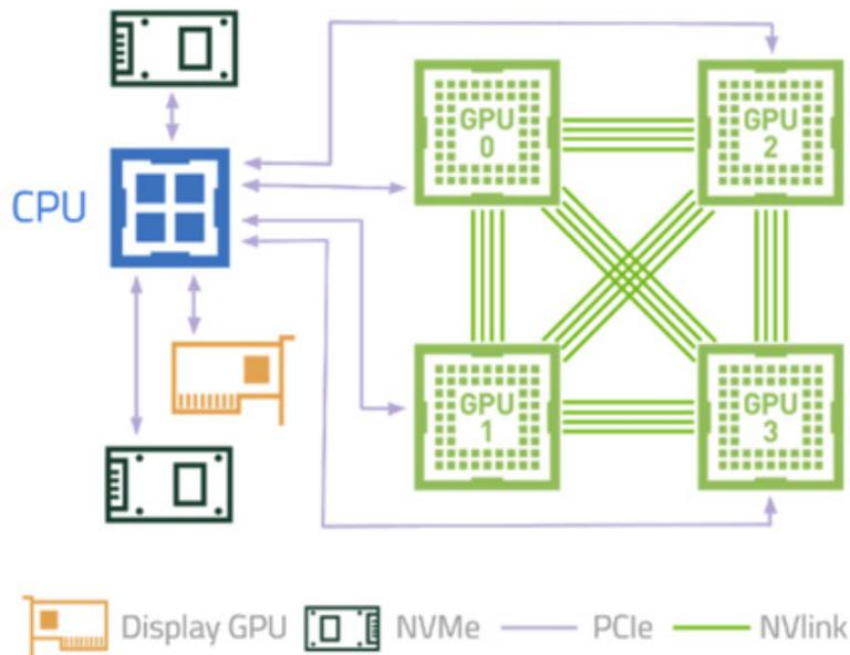
Figure 11. View of the DGX Station A100 devices topology
