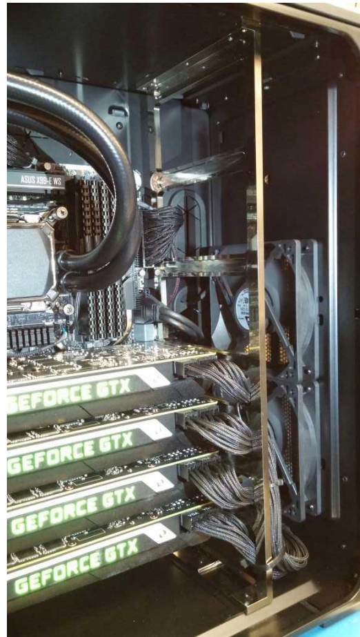
Figure 3. Custom Bracket to Support GPUs
