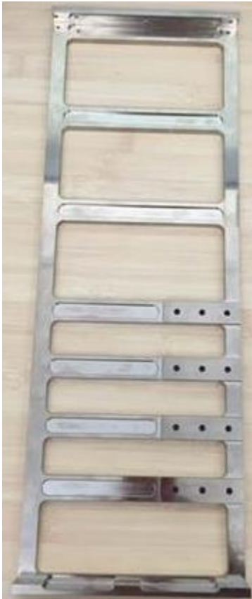
Figure 3. Custom Bracket to Support GPUs
