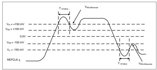
Figure 7. BCLK{0/1} Differential Clock Crosspoint Specification
