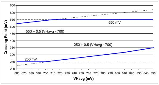
Figure 8. BCLK{0/1} Single Ended Clock Measurement Points for Absolute Cross Point and Swing
